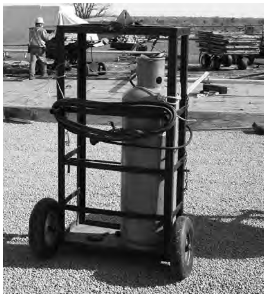
Upright Propane Tank Secured on Cart
