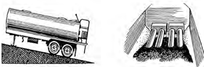
Setting Up Tanker on Slopes Creates Ideal Conditions for Fires
