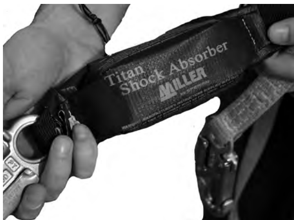
Check Cover Jacket for Stress or Tearing
