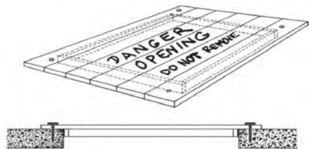
Protective Cover Over Opening
