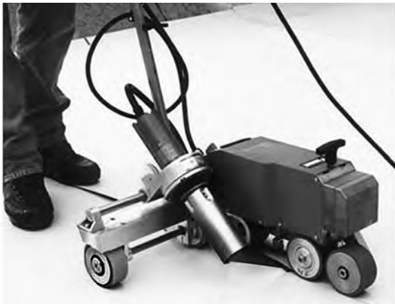
Roof Membrane Hot-air Welder
