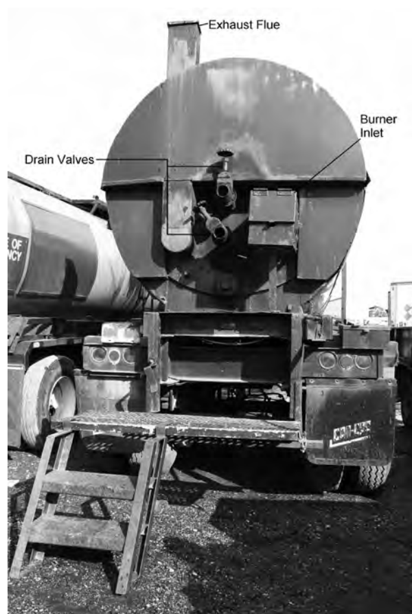
Tanker with Proper Access
