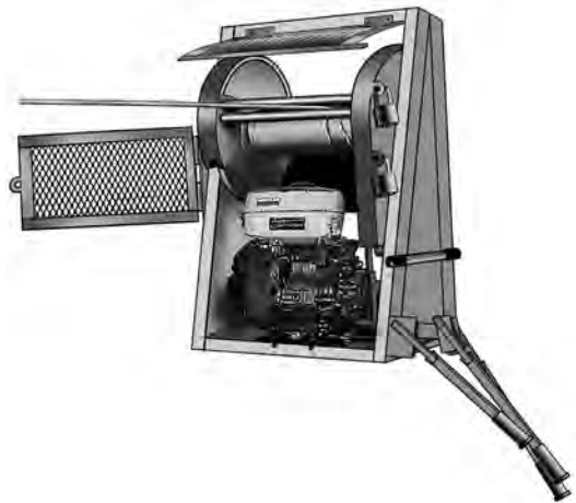
Figure 3: Cover with latch on the same side as the operator and hinge on opposite side
