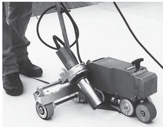
Roof membrane hot-air welder
